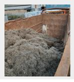
Bulk density 450 kg/m² Max load (RoRo) 13 tonne Wire diameter 0.2-0.8mm
